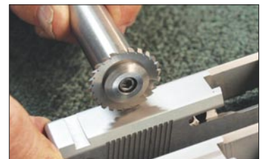
Showing cutting position for sight track
